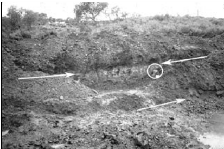
Figure 2. The color change (upper arrows) more than 1 foot above the gold pan (circled) marks the site of a pay streak in the drainage. This pay streak was probably produced during a flash flooding event, or during unusually high spring runoff. A second pay streak was found at the base of the open cut near the standing water (lower arrow). Even though this placer was essentially located in a dry drainage when mined, it was immediately downslope from some lode deposits, and provided a favorable site for gold concentration.
